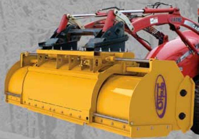
Snow plow with hydraulic panels 'S' and 'L' Category
